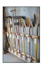
Cut PVC, drill holes and mount on to wood.
